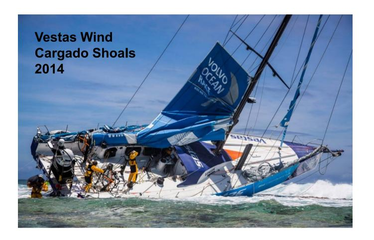
"Team Vestas Wind's grounding on the Cargados Carajos Shoals comes down to a basic failure in overall passage planning, and an over-reliance on electronic navigation."
