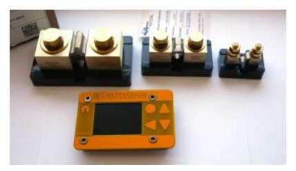
On the right side is the 10A 100mV Murata very similar to the RSA series and below the 200A and 100A 75mV inexpensive shunts.
