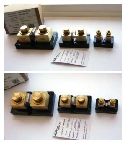
Not sure how clear this picture is (below), but the bottom screw heads are deep and will not touch the base you install this on and there is a clear resin on top of them.
